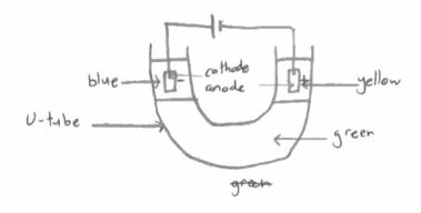
A & y-tube would be used in which the copper (11) chromate (VI) would be kept. At each end would be an electrode to pass a current through. The liquid is green, but after some time a blue toguide and yellow liquid will be seen at opposite electrods.
