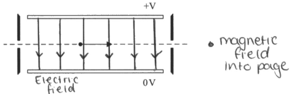
In one mass spectrometer the plates are 2.5 cm apart and a p.d. of 135 V is applied.
