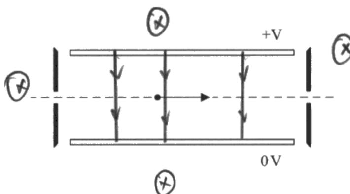
In one mass spectrometer the plates are 2.5 cm apart and a p.d. of 135 V is applied.
