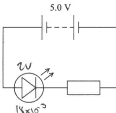
To be lit to normal brightness the current through the LED must be 18 mA.
