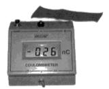
In a laboratory demonstration of the photoelectric effect, a sheet of zinc was placed on top of a coulombmeter and the zinc was given a negative charge.
