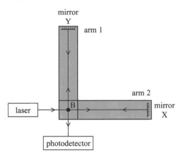
The laser beam is split into two at B, one beam travelling to one mirror and the other beam travelling to the other mirror. After reflection at the mirrors, the beams are recombined at B and reach the photodetector. The photodetector measures the intensity of the incident light.
