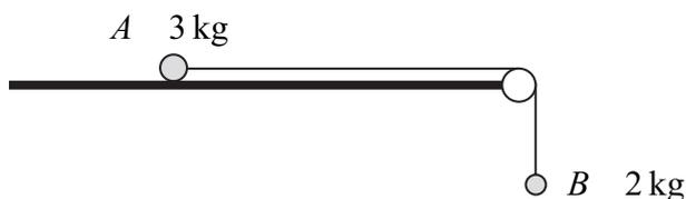
The particles are released from rest and move with a constant acceleration of magnitude  $0.9\text{ m s}^{-2}$ .
