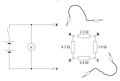
The four resistors are connected in a loop with sockets **A**, **B**, **C** and **D** at each junction. Two leads are used to connect the resistor loop to **X** and **Y**.
