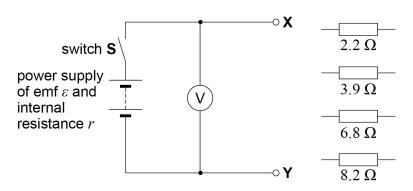
The student can change the external resistance R of the circuit between terminals  $\mathbf{X}$  and  $\mathbf{Y}$ . This is done by connecting different combinations of  $\mathbf{two}$  resistors in series or in parallel between  $\mathbf{X}$  and  $\mathbf{Y}$ .
