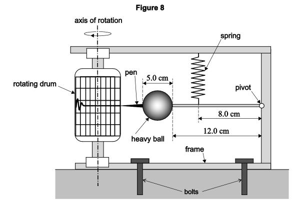
A heavy spherical ball is attached to a pivot by a rod so that the rod and ball can move in a vertical plane. The rod is suspended by a spring so that, in equilibrium, the spring is vertical and the rod is horizontal. A pen is attached to the ball. The pen draws a line on graph paper attached to a drum rotating about a vertical axis. Bolts secure the seismometer to the ground so that the frame of the seismometer moves during the earthquake.
