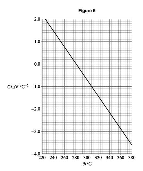
The neutral temperature  $\theta_n$  is the temperature corresponding to the maximum value of  $\varepsilon$ .  $\theta_n$  can be determined using either **Figure 5** or **Figure 6**.
