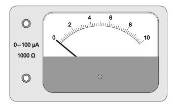
When this meter indicates a maximum reading and the needle points to the right-hand end of the scale (full-scale deflection), the current in the meter is  $100~\mu A$ . The meter has a resistance of  $1000~\Omega.$
