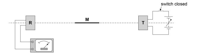
M is kept parallel to the marked line and moved slowly away as shown in Figure 3.
