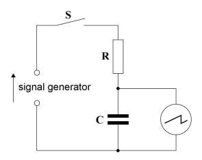
The oscilloscope is connected across the capacitor.
