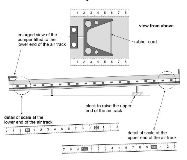
A glider is placed in contact with the rubber cord on the bumper at the lower end of the track. The position of the glider relative to the fixed scale can be determined using Figure 14.
